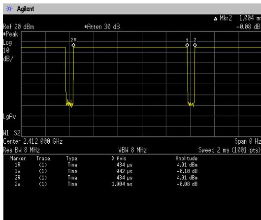
$$\text{Duty Cycle} = \text{Ton} / (\text{Ton} + \text{Toff}) = 942[\mu\text{s}] / (942[\mu\text{s}] + 62[\mu\text{s}]) = 93.82\%[ ]$$
