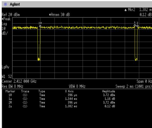
$$\text{Duty Cycle} = \text{Ton} / (\text{Ton} + \text{Toff}) = 1344[\mu\text{s}] / (1344[\mu\text{s}] + 38[\mu\text{s}]) = 97.25\%[ ]$$
