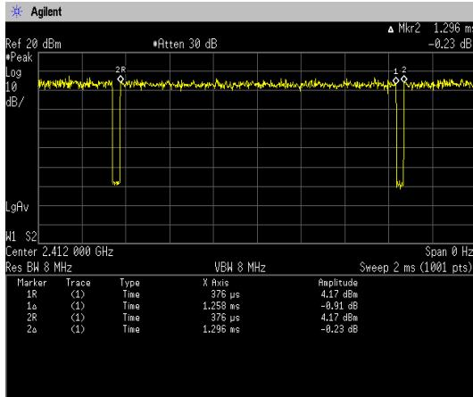
$$\text{Duty Cycle} = \text{Ton} / (\text{Ton} + \text{Toff}) = 1258[\mu\text{s}] / (1258[\mu\text{s}] + 38[\mu\text{s}]) = 97.07\%[ ]$$
