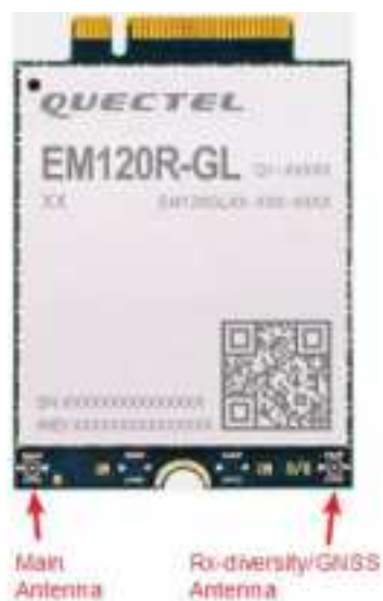
Figure 33: Antenna Connectors on the EM120R-GL Module
