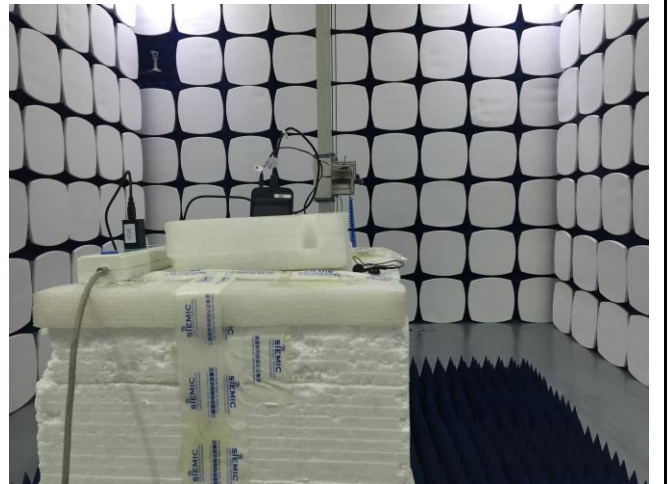
Radiated Spurious Emissions Test Setup Above 1GHz
