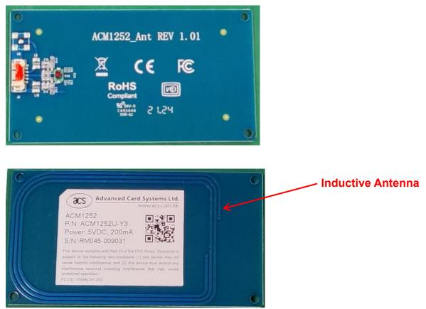
Note: The EUT has a printed antenna on PCB. which was permanently attached, the antenna gain is 0 dBi .
