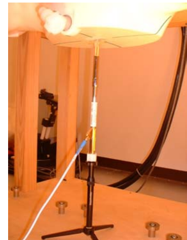
2450MHz System performance check setup
