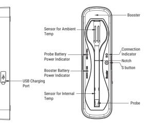
1. **Booster:** receives the temperature signal from the probe and boosts and transmits it to the smart device. It also serves as a power source to charge the probe.
