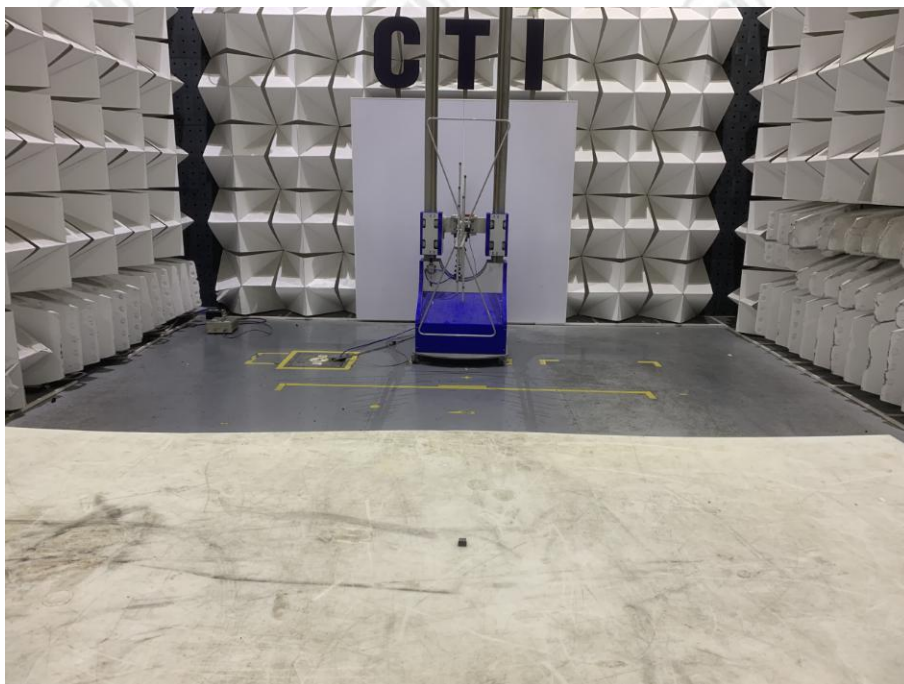
Radiated spurious emission Test Setup-1(Below 1GHz)
