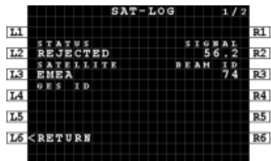
Figure 5-11: MCDU - SAT-LOG 1/2 - Status - Rejected
