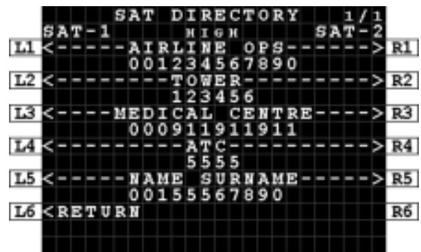
Figure 7-4: MCDU - SAT DIRECTORY X/Y
