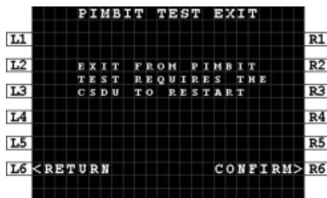
Figure 10-19: MCDU - BITE - PIMBIT - PIMBIT TEST RESULT - PIMBIT TEST EXIT
