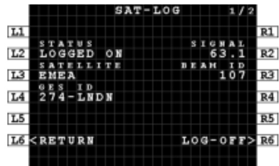
Figure 5-9: MCDU - SAT-LOG 1/2 - Status - Logged On
