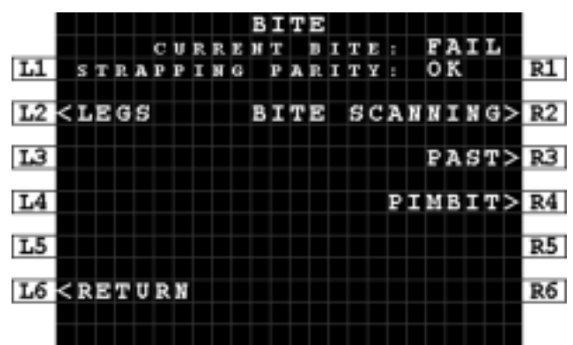
Figure 10-3: MCDU - BITE - FAIL
