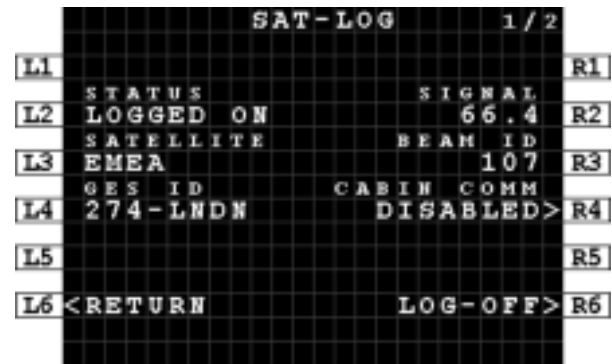
Figure 9-2: MCDU - SAT-LOG - Cabin Comm disabled
