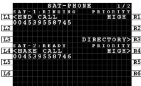
Figure 7-7: MCDU - SAT-PHONE 1/2 - Outgoing Call - Ringing
