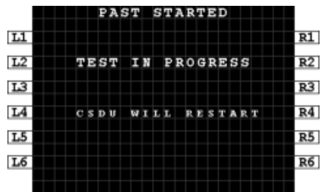
Figure 10-7: MCDU - BITE - PAST STARTED
