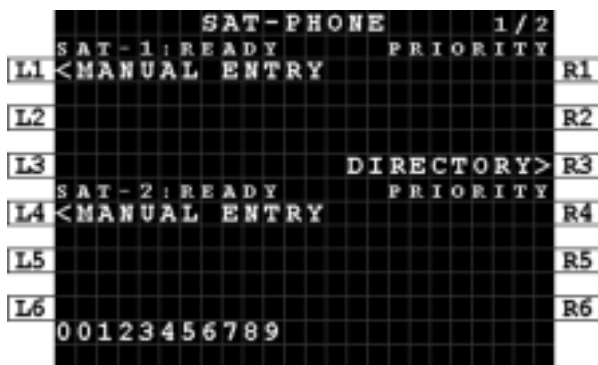
Figure 7-1: MCDU - SAT-PHONE 1/2 - Manual Entry - International Number - Scratchpad
