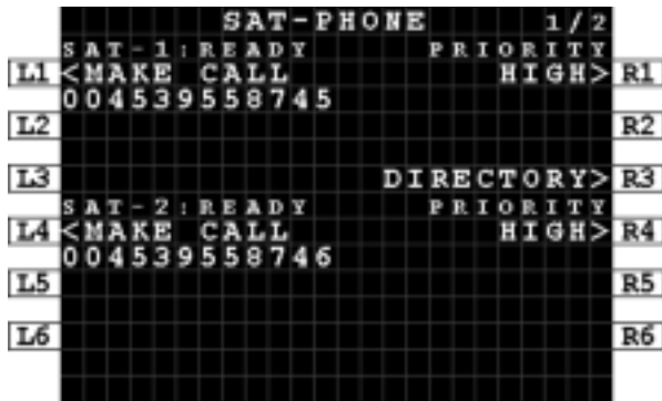
Figure 7-5: MCDU - SAT-PHONE 1/2 - Outgoing Call - Make Call
