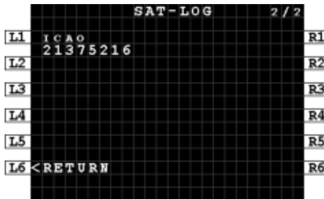
Figure 5-13: MCDU - SAT-LOG 2/2 - ICAO
