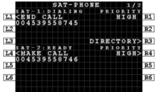
Figure 7-6: MCDU - SAT-PHONE 1/2 - Outgoing Call - Dialing
