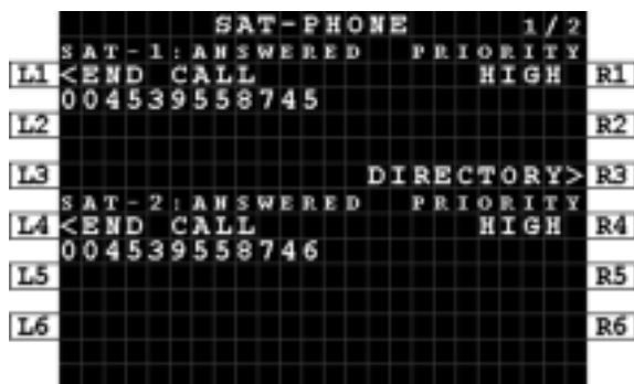
Figure 7-10: MCDU - SAT-PHONE - Ending a call
