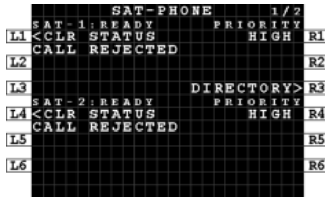
Figure 7-15: MCDU - SAT-PHONE - Incoming Call - Rejected
