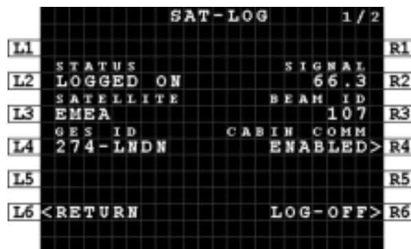
Figure 5-6: MCDU - SAT-LOG 1/2 - Safety Data Available
