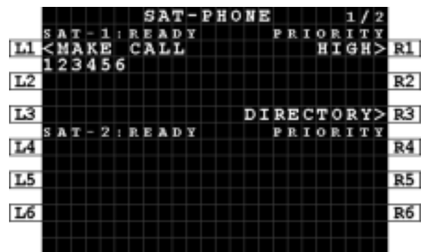
Figure 7-2: MCDU - SAT-PHONE - Manual Entry - Short Code - Pre-selected
