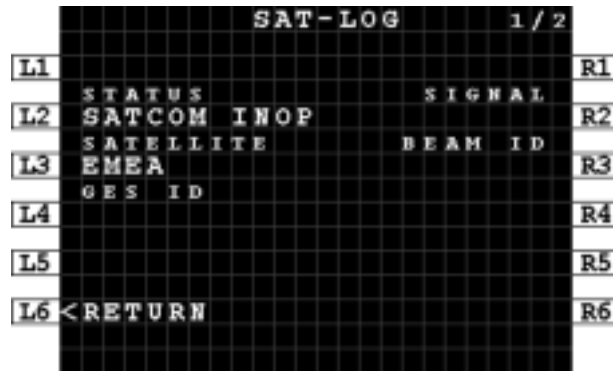
Figure 5-12: MCDU - SAT-LOG 1/2 - Status - SATCOM INOP
