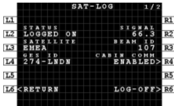
Figure 8-1: MCDU - SAT-LOG - ACARS Data Available
