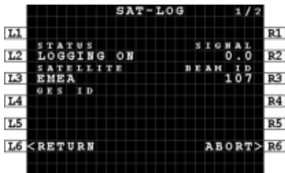
Figure 5-8: MCDU - SAT-LOG 1/2 - Status - Logging On
