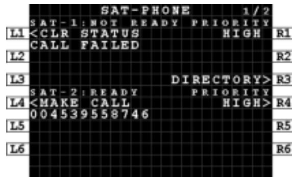
Figure 7-9: MCDU - SAT-PHONE 1/2 - Outgoing Call - Call Failed
