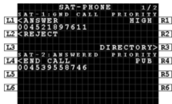
Figure 7-17: MCDU - SAT-PHONE - Incoming Call - Preemption Caller ID
