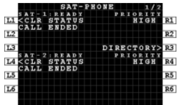
Figure 7-11: MCDU - SAT-PHONE - Call ended
