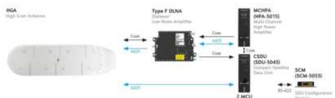
Figure 3-2: AVIATOR 700S SATCOM System
