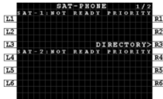
Figure 5-3: MCDU - SAT-PHONE 1/2 - NOT READY
