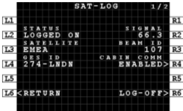
Figure 9-1: MCDU - SAT-LOG- Cabin Comm enabled
