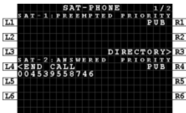
Figure 7-16: MCDU - SAT-PHONE - Incoming Call - Preempted
