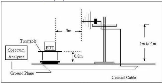
(C) Radiated Emission Test-Up Frequency Above 1GHz
