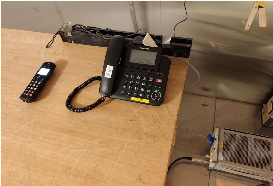
Power-Line Conducted Emissions Test
