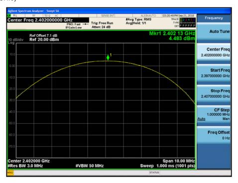
Test Plots (π/4DQPSK) Peak Power (CH.39)
