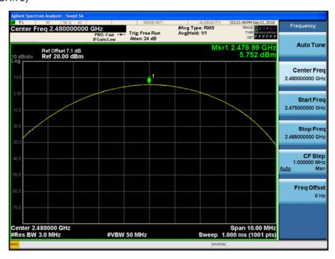
Test Plots (π/4DQPSK) Peak Power (CH.0)
