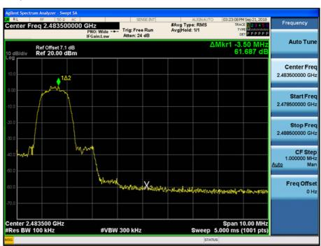
Test Plots with hopping (GFSK) Band Edges (CH.0)
