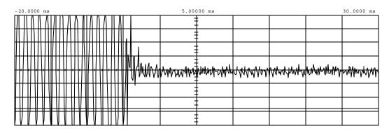
Trigger mode : Edge On Negative Edge Of Chan2 Trigger Level Chan2 = -27.500 mV (noise reject ON) Holdoff = 40.000 ns
