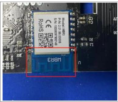
The antenna is PCB antenna. The best case gain of the antenna is 2.5 dBi.
