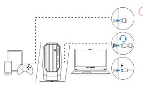
Plug the USB C dongle to USB C port on your computer or Plug the USB wireless dongle into the A to C adaptor, and then connect the adaptor to the USB A port on your computer.
