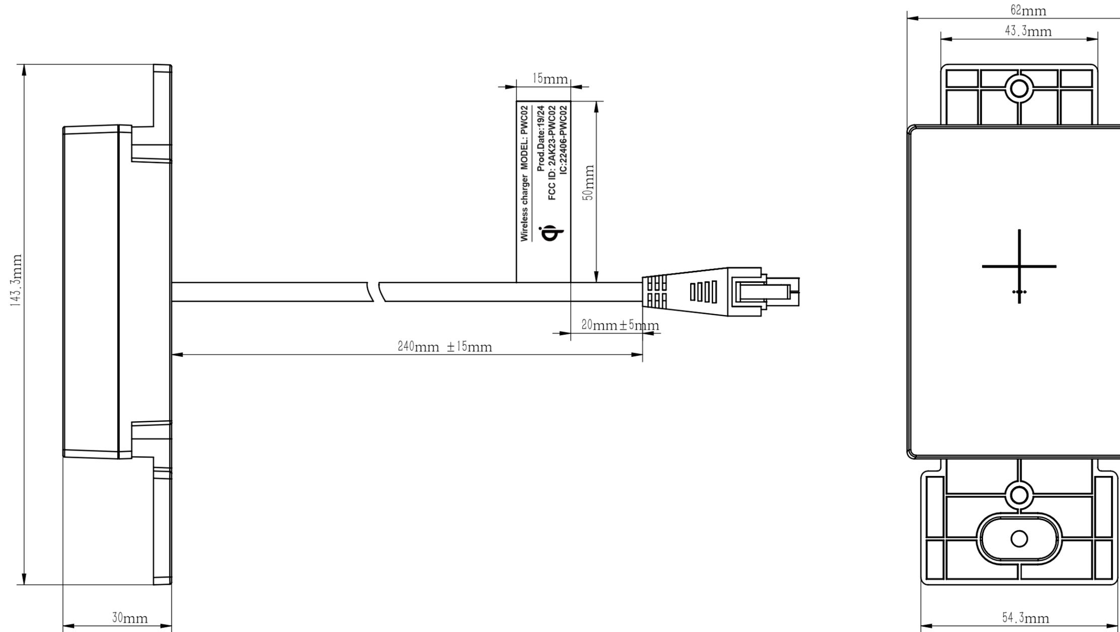
Note: This label is made of PET material and fixed on the cable in the form of solid adhesive, so that it will not fall off during the expected life of the product.
