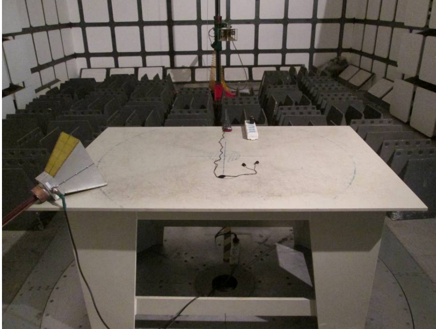
Radiated Emissions –Front View (1-25 GHz)
