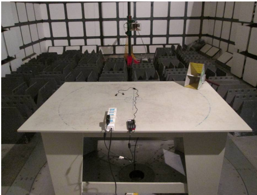
Radiated Emissions –Rear View (1-25 GHz)
