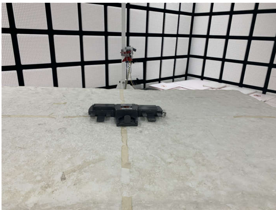
Radiated spurious emission Test Setup-2(Above 1GHz)
