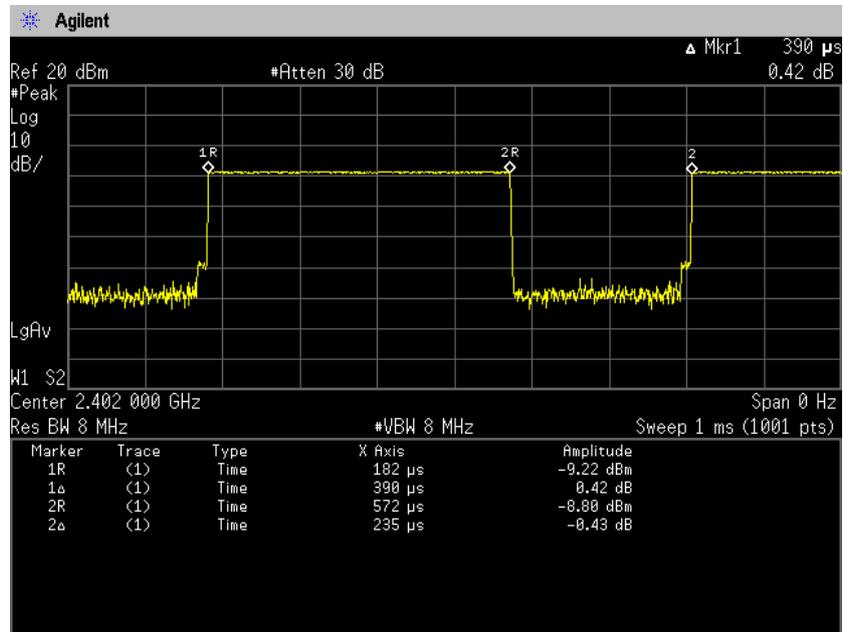
$$\text{Duty Cycle} = T_{\text{on}} / (T_{\text{on}} + T_{\text{off}}) = 390[\mu\text{s}] / (390[\mu\text{s}] + 235[\mu\text{s}]) = 62.4[\%]$$
