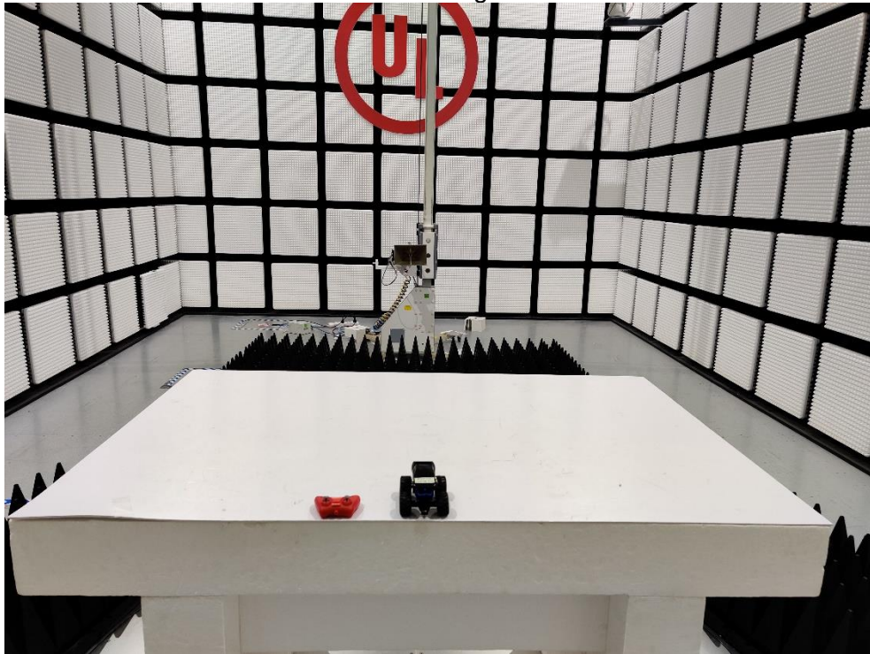
Radiated Emissions above 1GHz test setup photo
