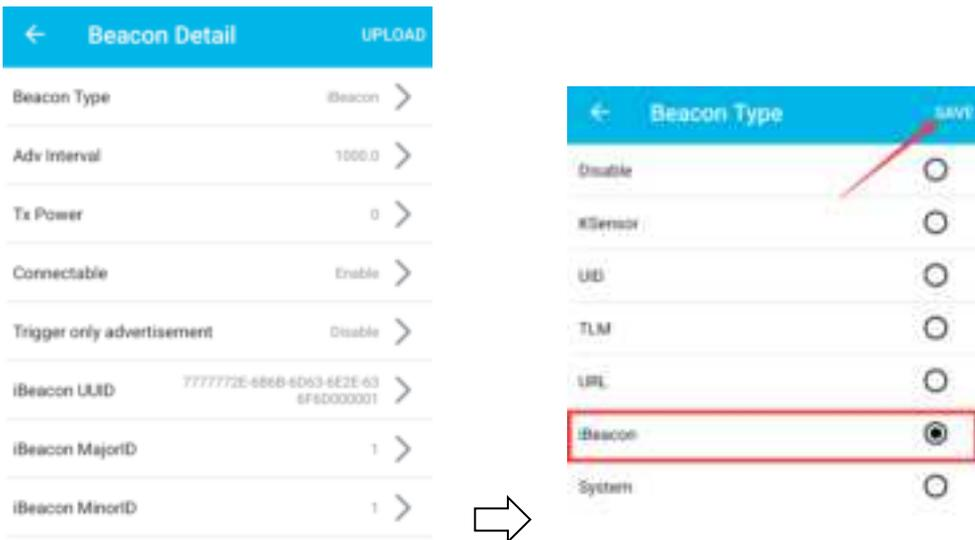
iBeacon parameters (UUID, Major ID, Minor ID, Adv Interval, TX power etc.) can also be configured in the App. Eddystone URL, UID, TLM, can be configured by the same steps above.
