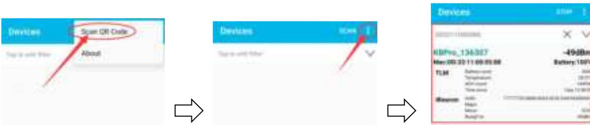
Reminder: iOS App filter the device by Device Name when use the ‘Scan QR code’ method. If the device name is not KBPro, the device can not be found on iOS App when scan the QR code.
