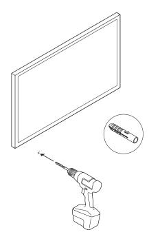
3. If you're using wall anchors, use a 5/16" drill bit to drill pilot holes, starting with the hole on the left. Then insert the wall anchors. Don't use wall anchors if you're drilling into wood or plastic (see **Wall mounting information**).
