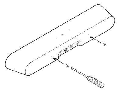
**5.** Using a Phillips head screwdriver, fasten the 2 attachment screws to the back of the soundbar, making sure they are fully tightened.
