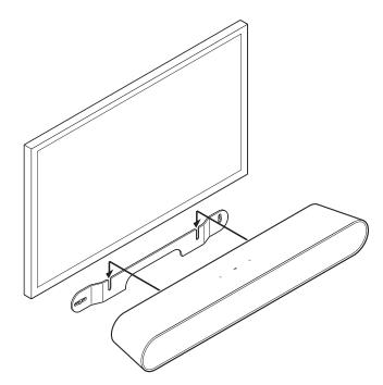
7. Slide the soundbar down so the attachment screws fit into the slots on the wall bracket.
