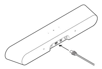
**6.** Remove the protective cap from the optical cable, then connect the power and optical cables to the back of the soundbar.
