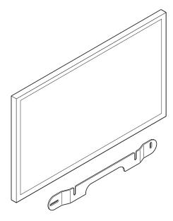
1. If your TV is wall-mounted, align the top edge of the bracket with the bottom of your TV, leaving at least 2.5 inches (mm) between them.
