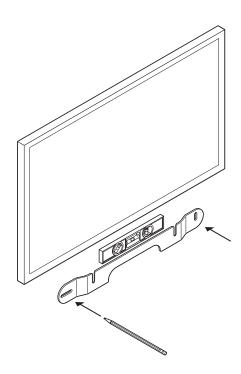
2. Mark the screw locations and remove the bracket.
