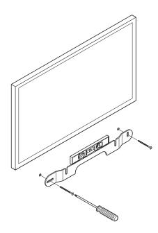
**4.** Position the wall mount bracket over the screw locations, using a level to confirm accuracy. Use a Phillips-head screwdriver or a power drill to screw the bracket to the wall, making sure the center notch is pointing up.
