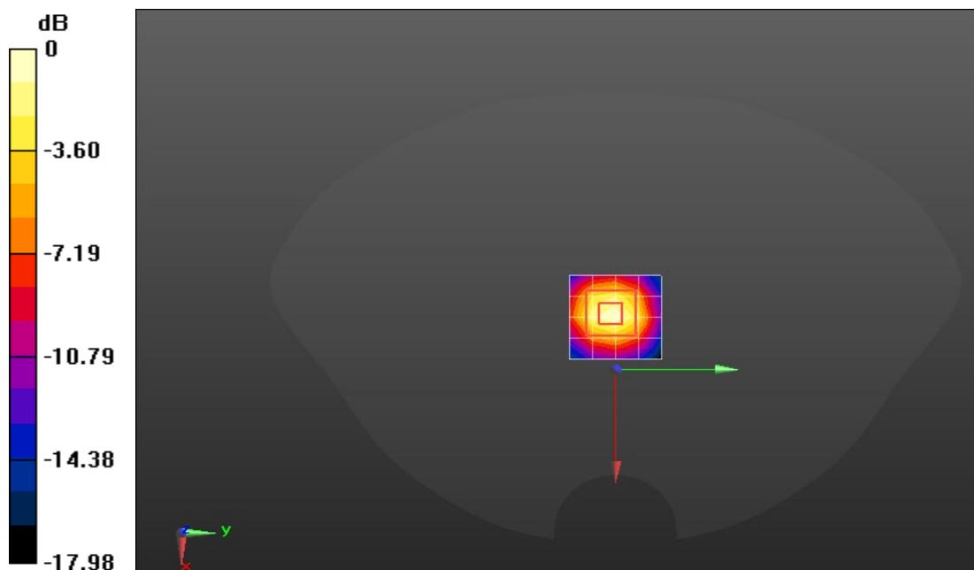
$$0 \text{ dB} = 8.88 \text{ W/kg} = 9.48 \text{ dBW/kg}$$
