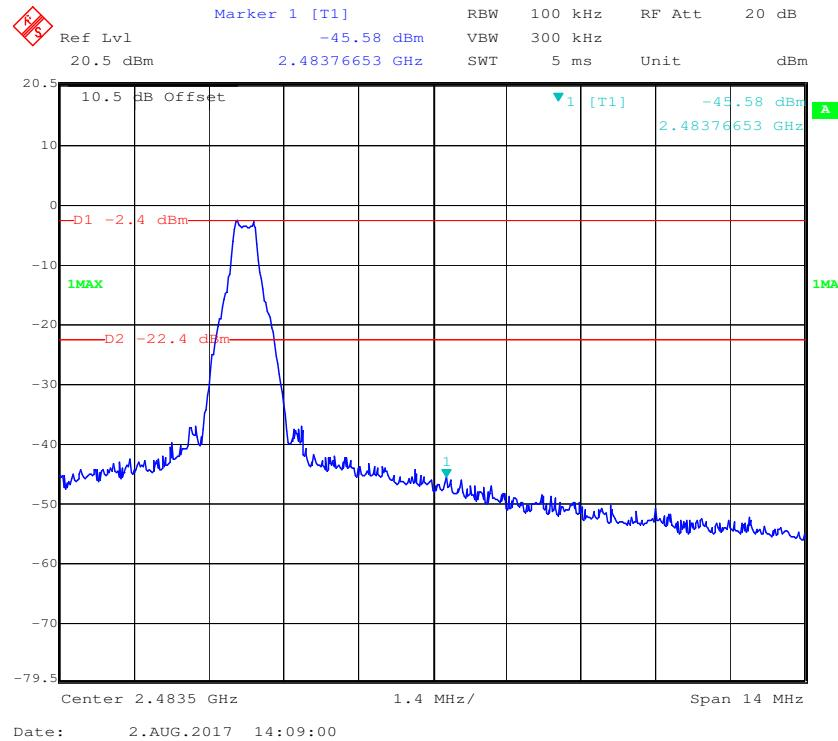
**EDR ( $\pi/4$ -DQPSK): Band Edge-Left Side**
