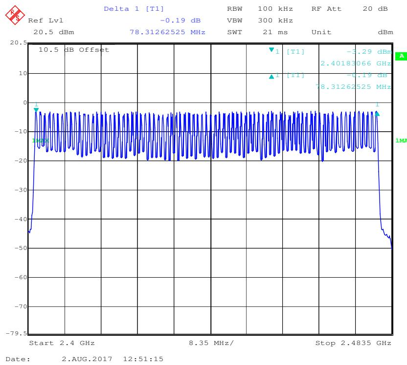
**EDR ( $\pi/4$ -DQPSK): Number of Hopping Channels**
