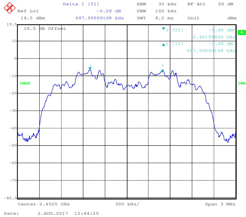
**EDR ( $\pi/4$ -DQPSK): Middle Channel**
