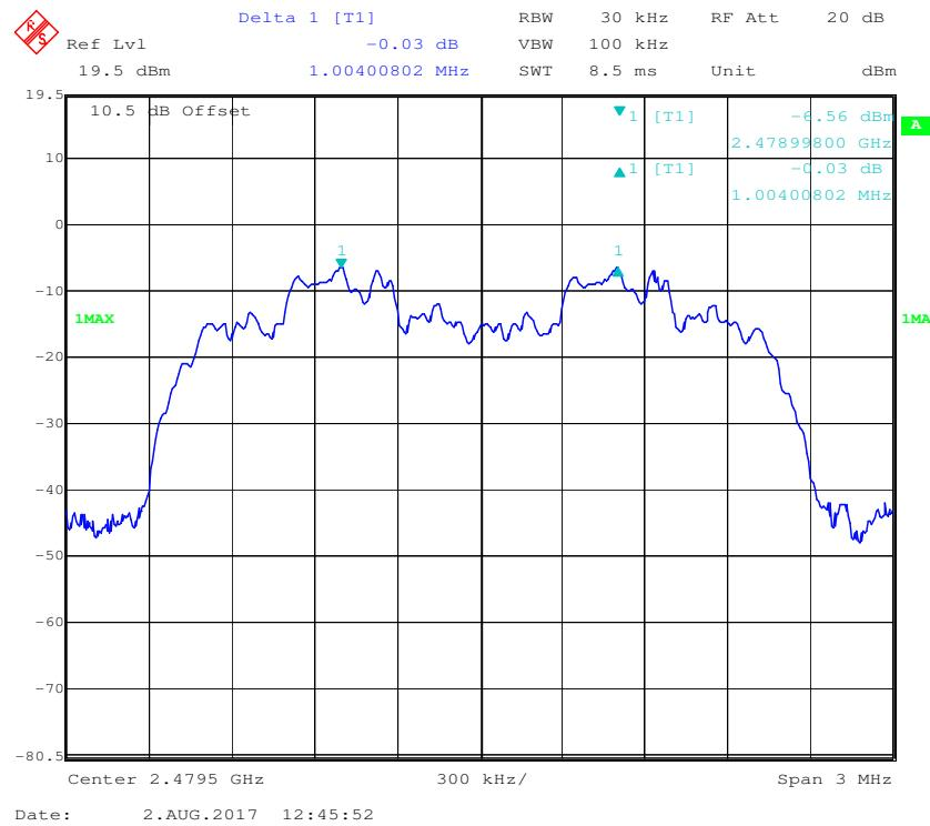
**EDR (8DPSK): Low Channel**
