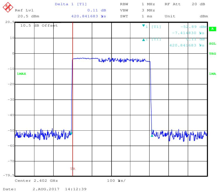
**Pulse time, Middle Channel, 2DH1**
