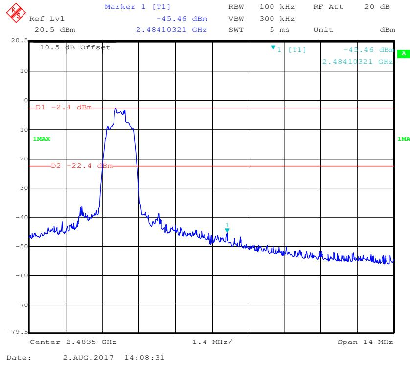
**EDR (8DPSK): Band Edge-Left Side**
