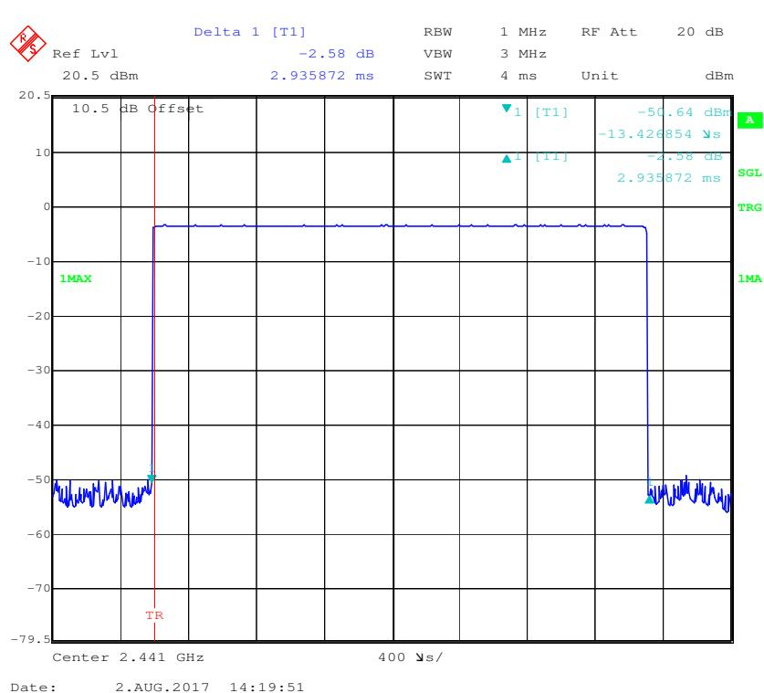
**Pulse time, High Channel, DH5**
