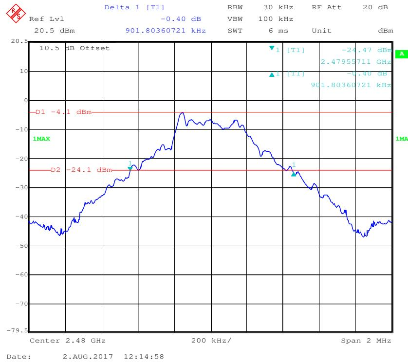
**EDR ( $\pi/4$ -DQPSK): Low Channel**
