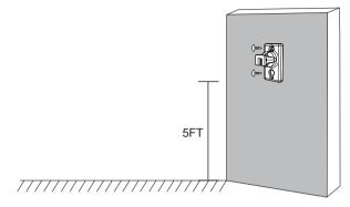
1.Install the transmitter mounting bracket in the desired location with the included screws.
