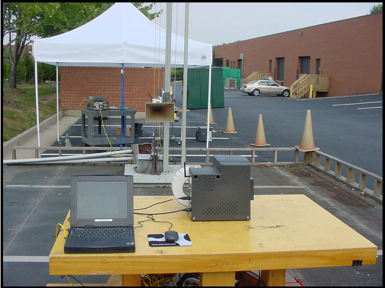
PHOTOGRAPH 3: RADIATED EMISSION FRONT VIEW; WORST CASE CONFIGURATION
