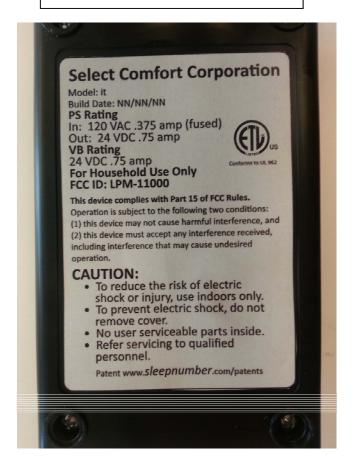
The label is placed on the back side of the enclosure for the WiFi Radio
