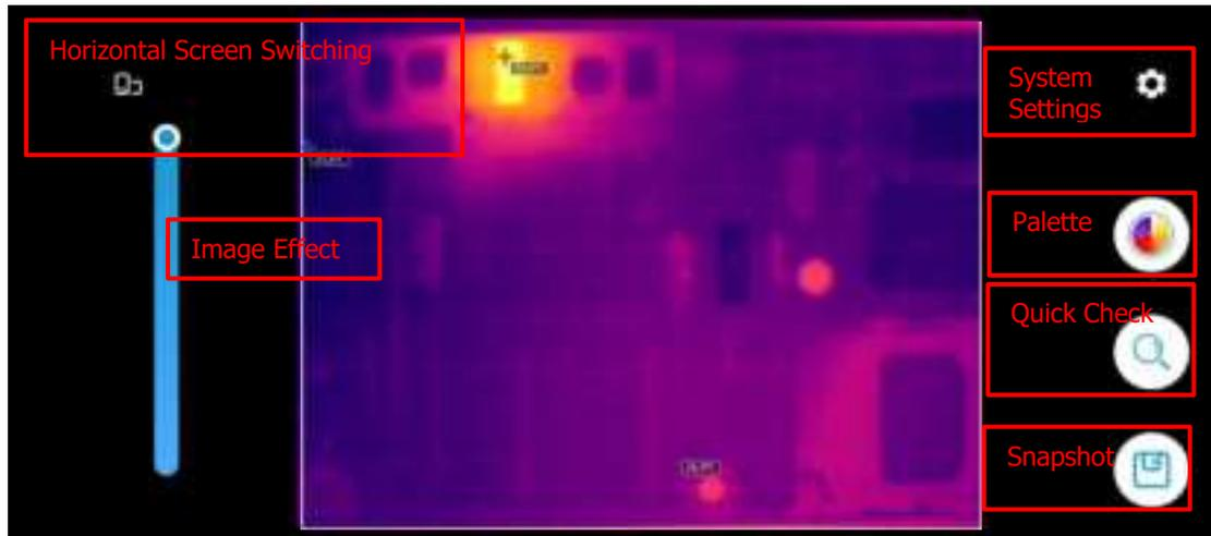
**App function buttons are as follows, the function is the same as the PC client software:**
