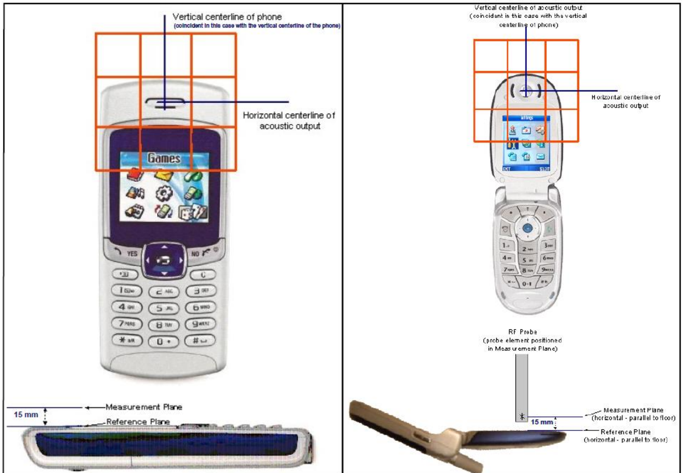
Fig-3.4 EUT Reference and Plane
