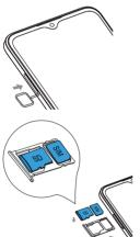
Insert the SIM pin that's provided to eject the SIM tray and then slide it out gently.
