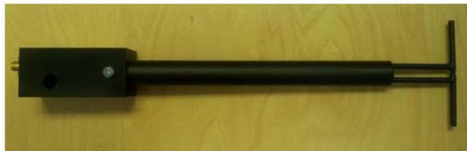
Figure 1 – MVG COMOSAR Validation Dipole
