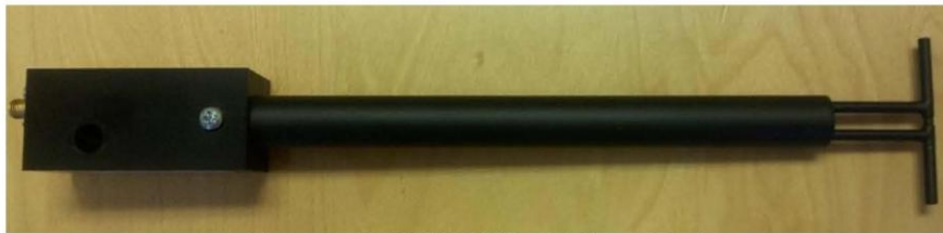
Figure 1 – MVG COMOSAR Validation Dipole
