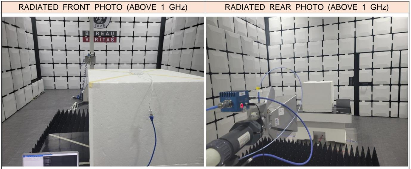
**RADIATED RF MEASUREMENT SETUP (18 - 26.5 GHz) X axis**
