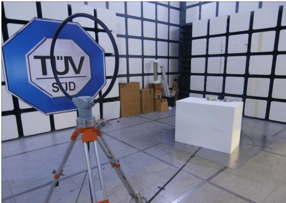
Figure 9 - Test Setup - 9kHz to 30MHz
