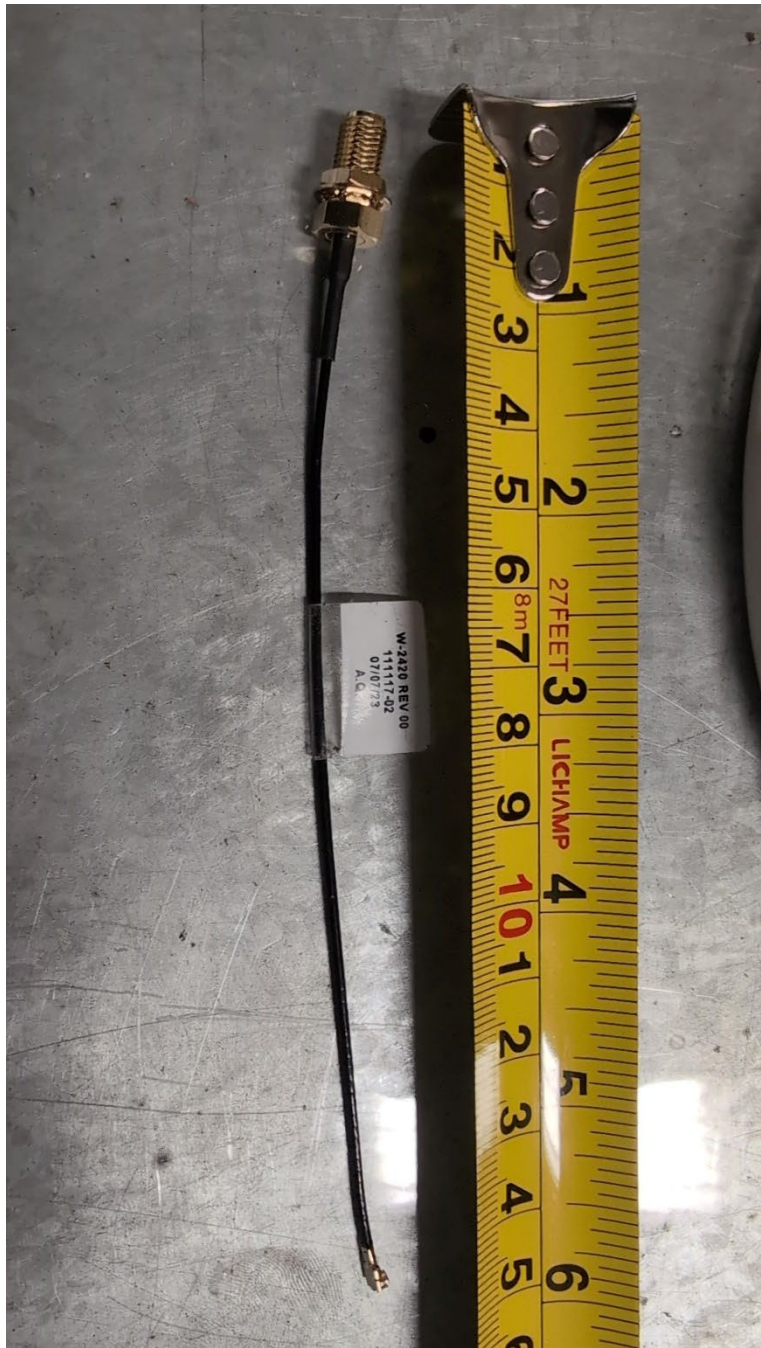
Reverse polarity SMA to U.FL cable
