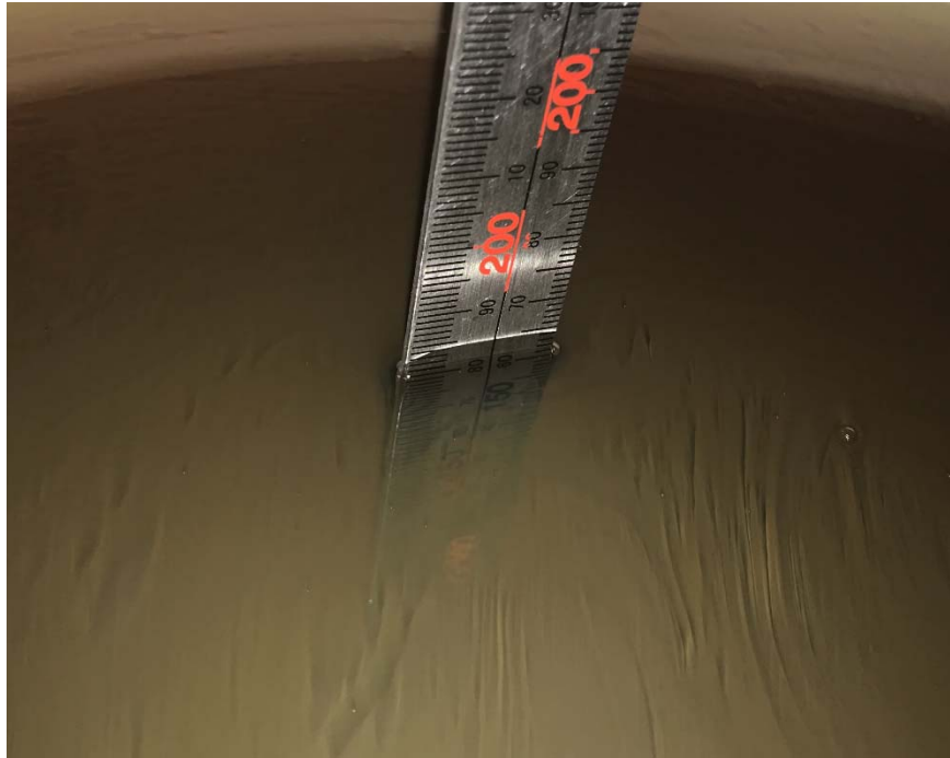
Liquid depth for SAR Measurement
