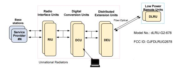
The matched units RIU/DCU/DEU are unintentional radiators, the fiber used to connect dLRU, DCU and DEU.
