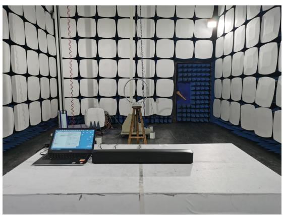
3. Radiated emission (9KHz-30MHz)
