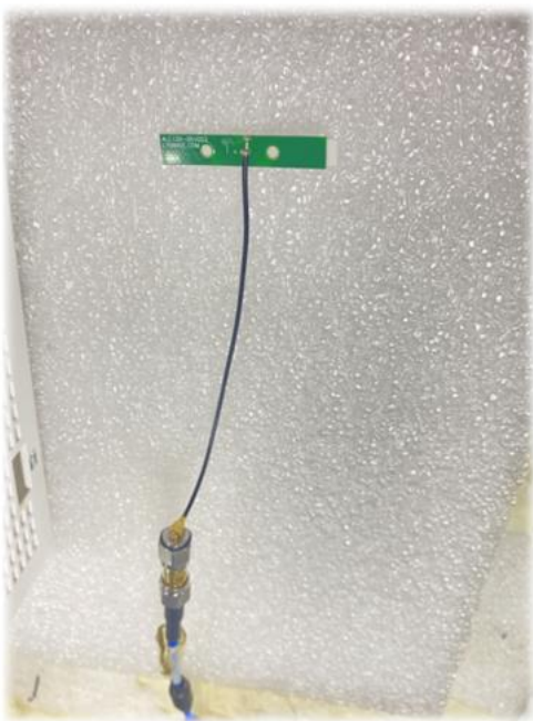
Antenna tested in free space
