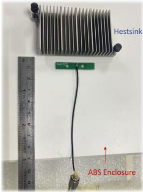
Antenna tested with ABS Antenna is 5mm away from metal
