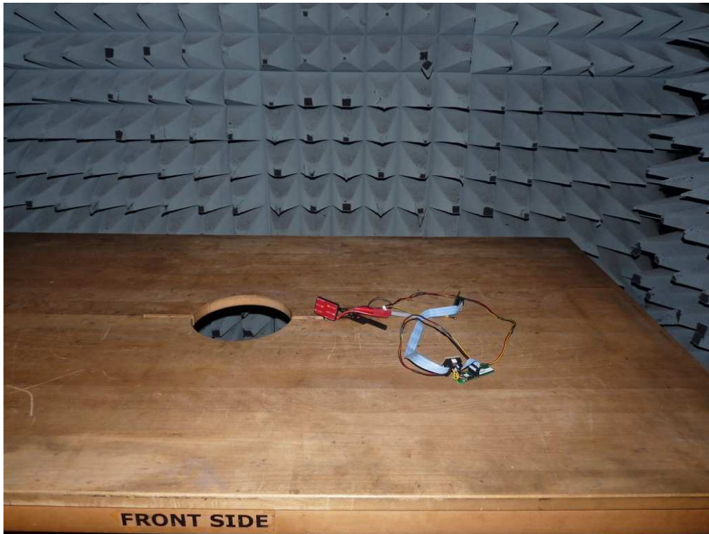
Photo 1: Test setup for radiated measurements (below 30 MHz)
