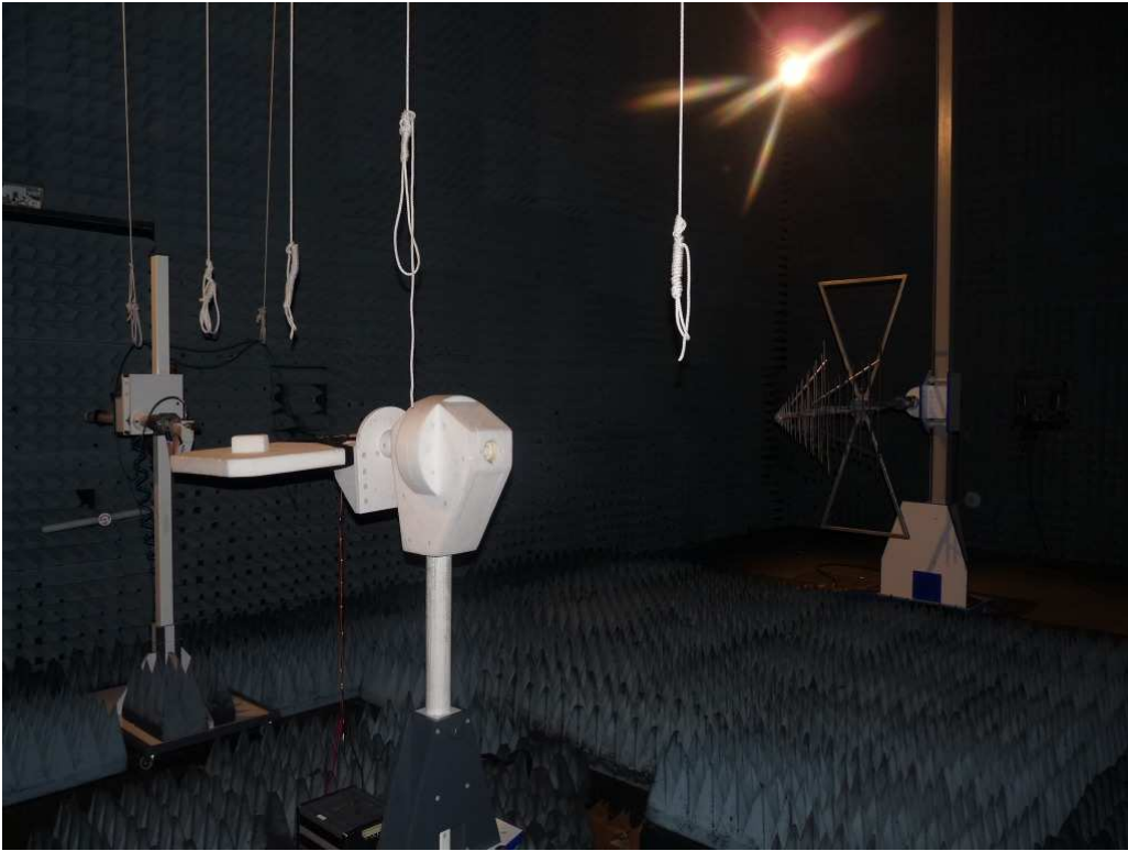
Photo 4: Test setup for radiated measurements (18 GHz up to 25 GHz)
