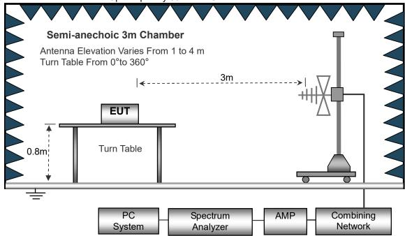
(C) Radiated Emission Test-Up Frequency Above 1GHz
