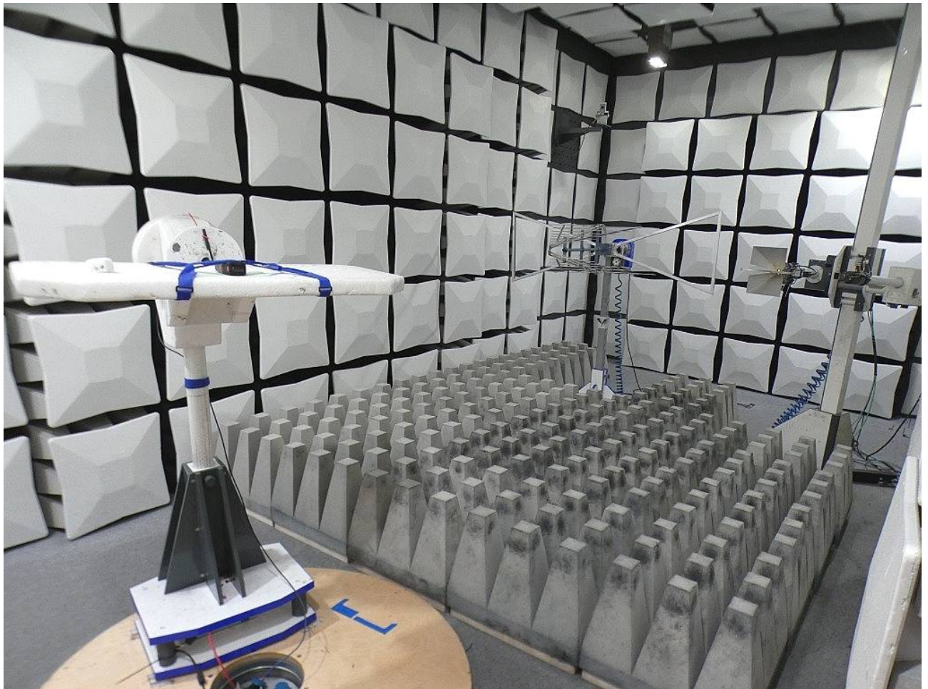
Photo 3: Test setup for radiated measurements (Enclosure, fully anechoic chamber, 1-26 GHz intentional radiator §15.209, ANSI C63.10)
