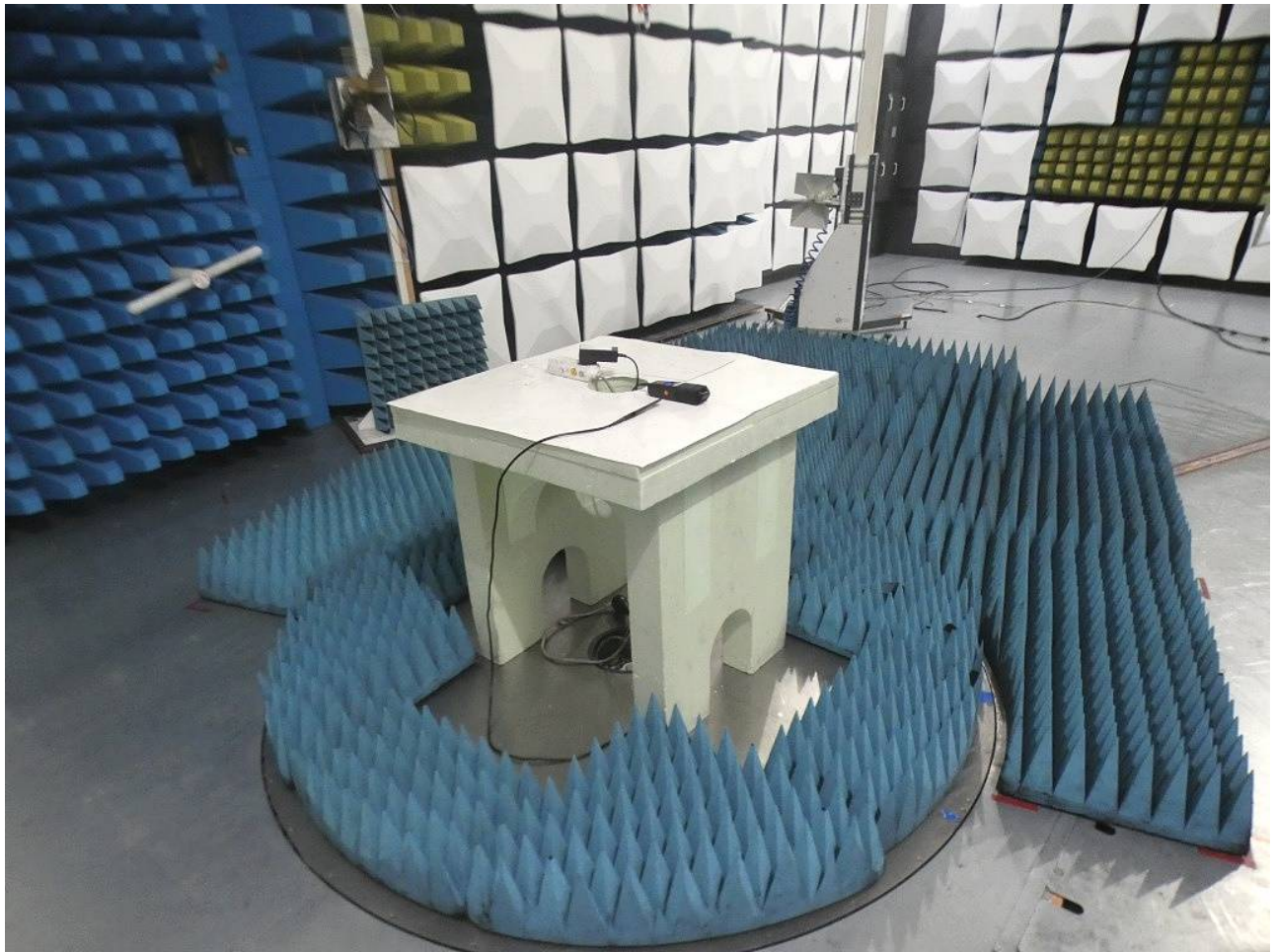
Photo 8: Test setup for radiated measurements (EUT supplied by AC/DC adapter, 1–12.5 GHz, unintentional radiator §15.109, ANSI C63.4, boresight mast)
