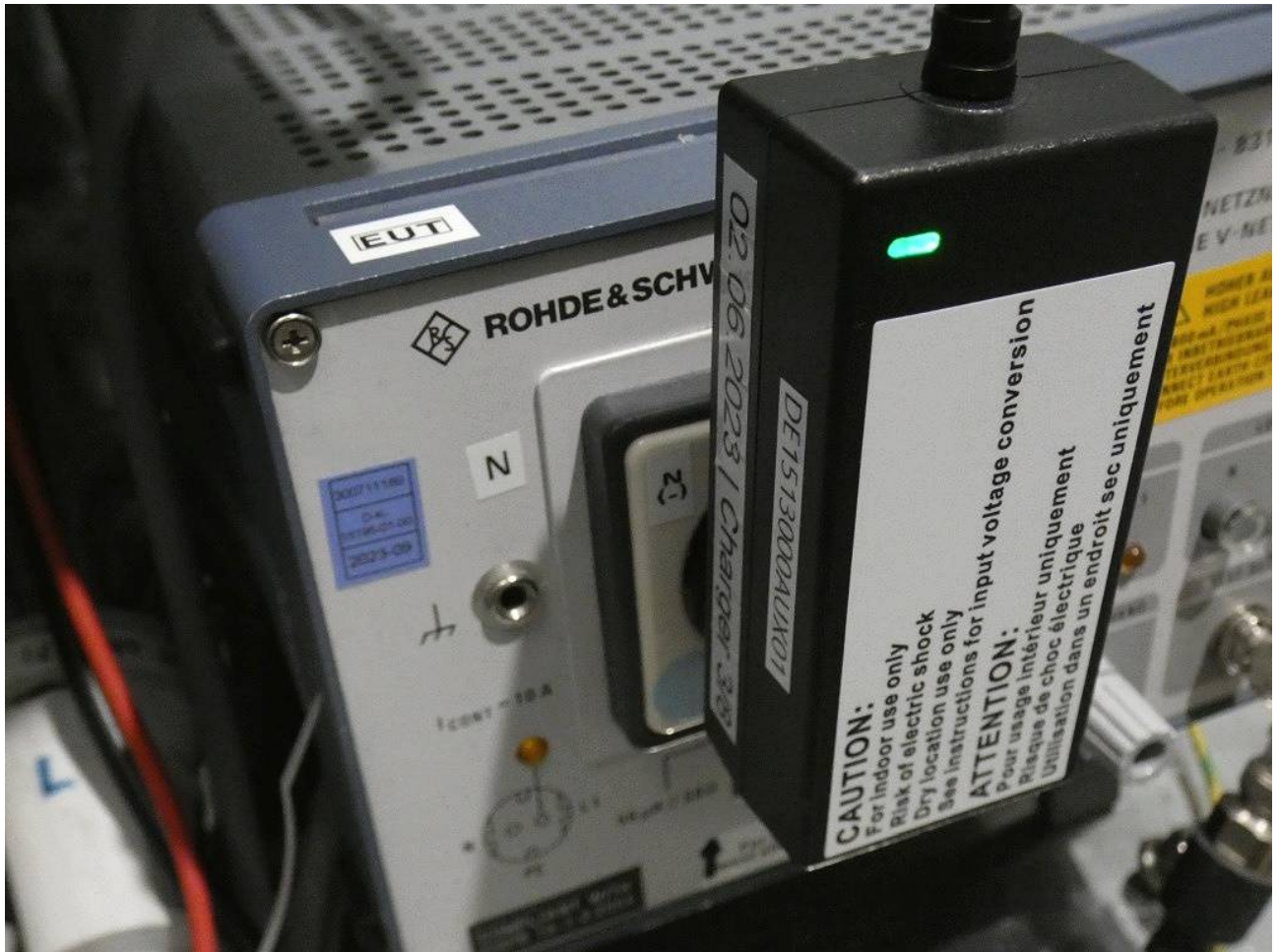
Photo 5: Test setup for conducted measurements (AC Port (power line), EUT supplied by AC/DC adapter, intentional / unintentional radiator §15.107/207, ANSI C63.4/10) arrangement of AC adapter
