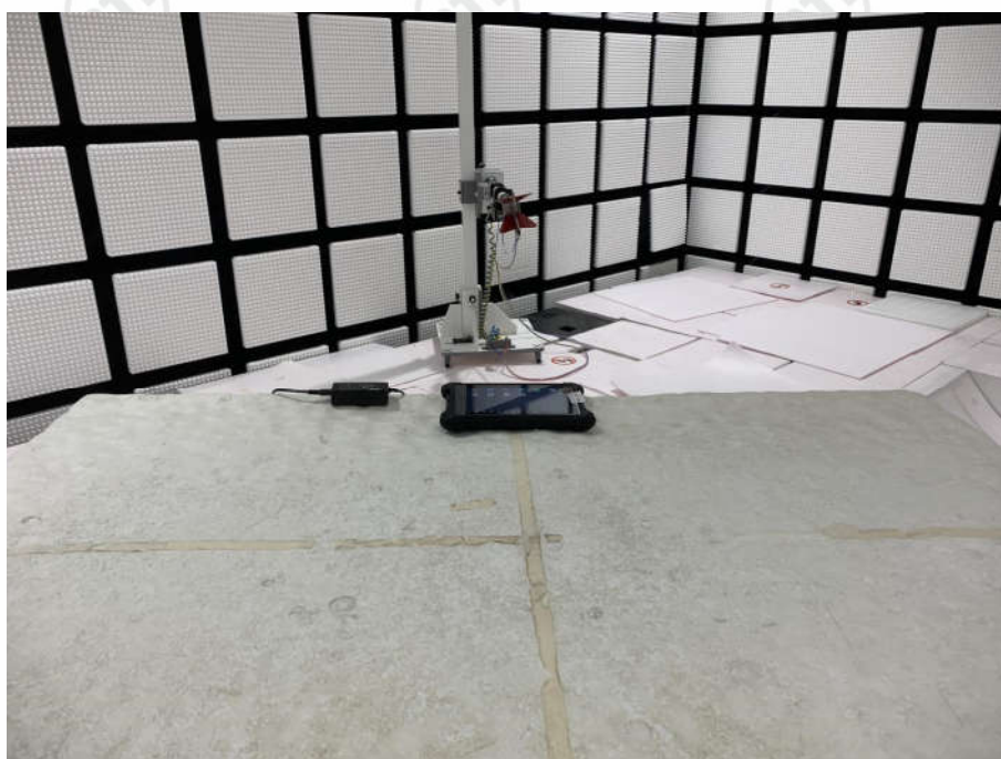
Radiated spurious emission Test Setup-2(Above 1GHz)
