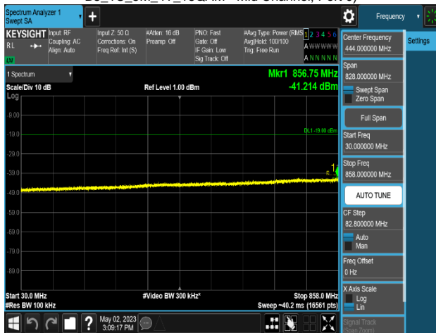
Plot 8-720. Conducted Spurious Emission Plot 30 MHz to 858 MHz (MSR 3C_DSS B(n)5_1C_10M+NR n5_1C_10M+LTE B5_1C_5M_4T_16QAM - Mid Channel, Port 0)
