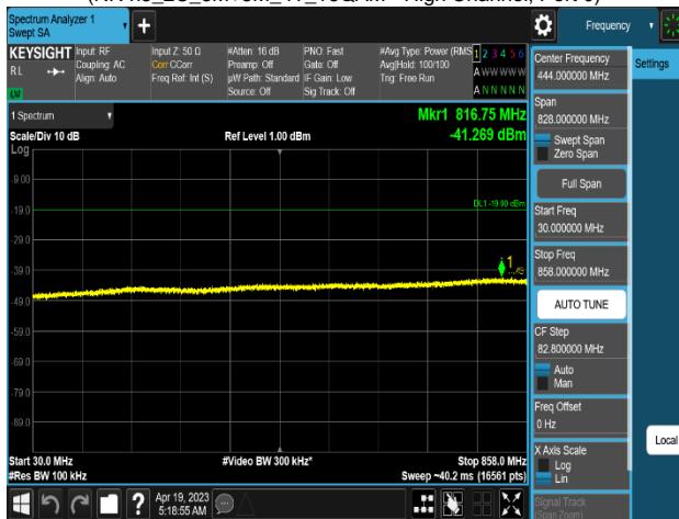
Plot 8-678. Conducted Spurious Emission Plot 30 MHz to 858 MHz
