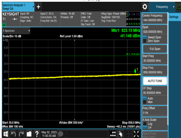
Plot 8-714. Conducted Spurious Emission Plot 30 MHz to 858 MHz (MSR 2C_NR n5_1C_5M+LTE B5_1C_5M_4T_QPSK - Low Channel, Port 0)
