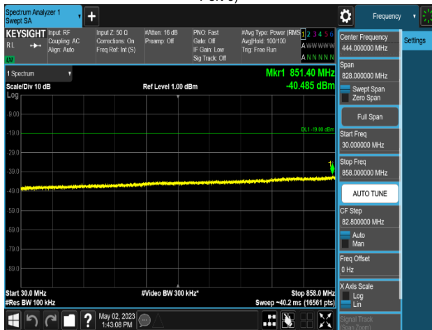
Plot 8-726. Conducted Spurious Emission Plot 30 MHz to 858 MHz (MSR 2NC_NR n5_1C_5M+LTE B5_1C_5M_4T_QPSK - Mid Channel, Port 0)
