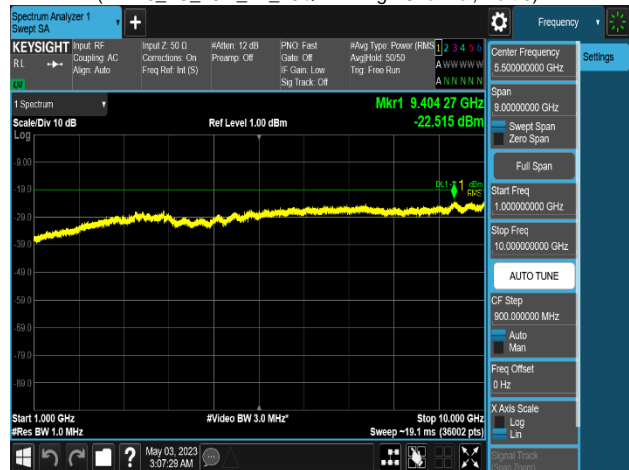
Plot 8-675. Conducted Spurious Emission Plot 1 GHz to 10 GHz (NR n5_1C_15M_4T_16QAM - High Channel, Port 0)
