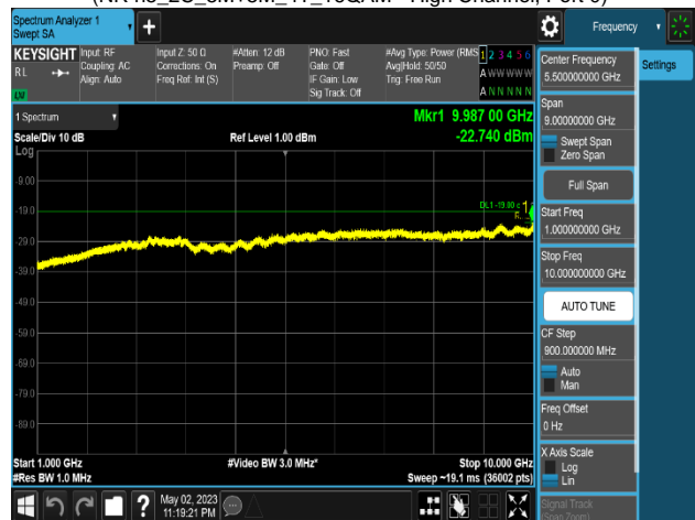
Plot 8-681. Conducted Spurious Emission Plot 1 GHz to 10 GHz
