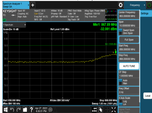
Plot 8-697. Conducted Spurious Emission Plot 858 MHz to 868 MHz (MSR 2C_DSS B(n)5_1C_10M+LTE B5_1C_5M_4T_QPSK - High Channel, Port 0)
