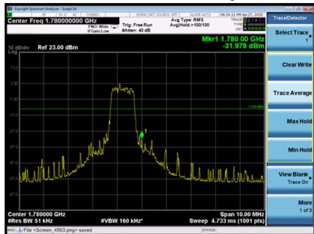
LTE Band 66 16QAM 5MHz CH-High, 1 RB
