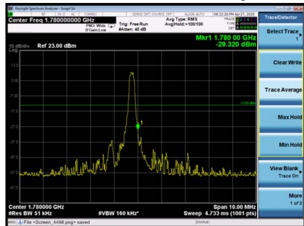
LTE Band 66 16QAM 1.4MHz CH-High, 100%RB
