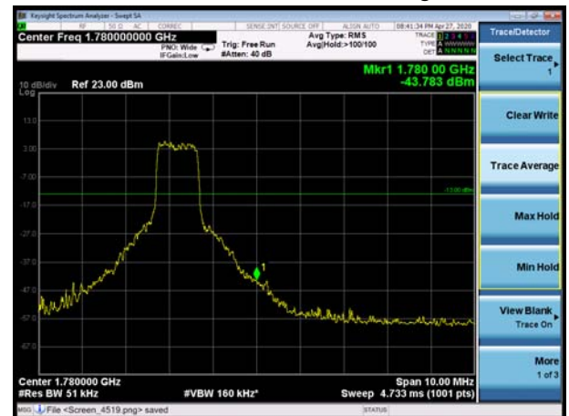
LTE Band 66 16QAM 20MHz CH-High, 100%RB
