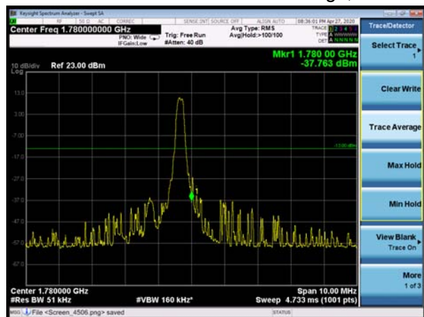
LTE Band 66 16QAM 5MHz CH-High, 100%RB
