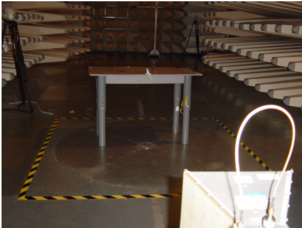
Set-up for Radiation Emission (Transceiver)
