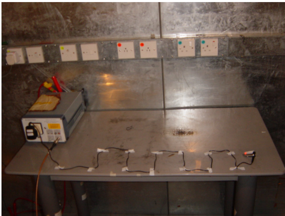
Set-up for Disturbance voltage on AC mains
