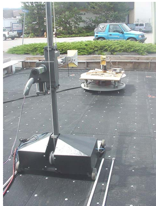
Photograph B.7-4 - Horn Substitution Setup
