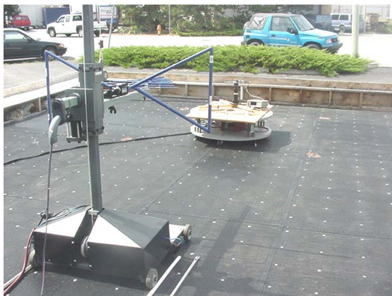
Photograph B.7-3 - Dipole Substitution Setup
