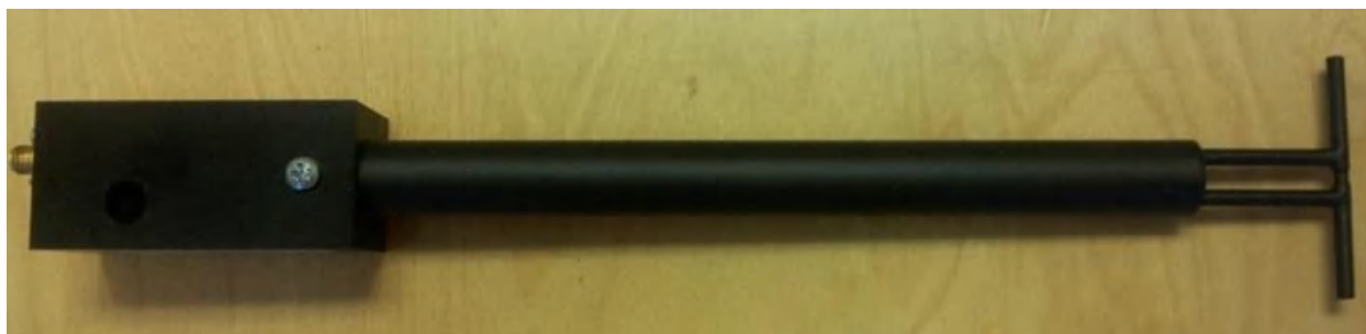
Figure 1 – MVG COMOSAR Validation Dipole
