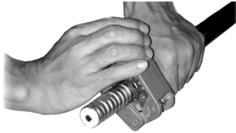
Fig. 10.4-7 Cutting the Feeder with a Cutter
