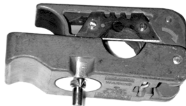
Fig. 10.4-6 Cutting Tool for the 7/8" Feeder Connector
