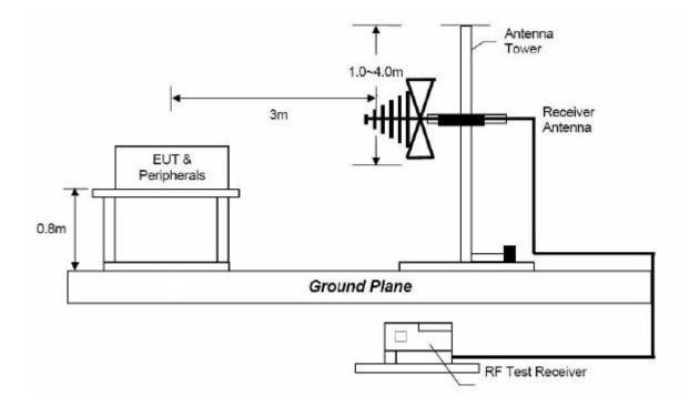
Radiated Emission Test Set-Up, Frequency above 1GHz
