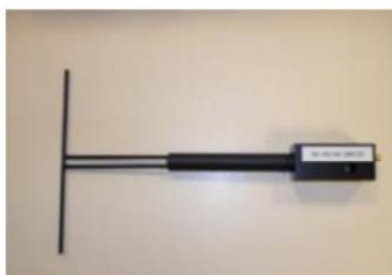
Figure 1 – Satimo COMOSAR Validation Dipole
