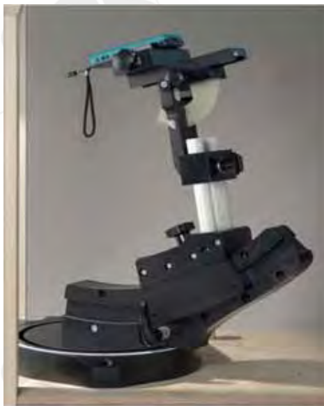
F-2. Device Holder for Transmitters
